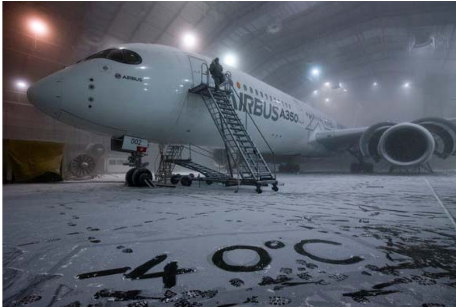
Figure 37 Airbus A350 at the McKinley Climatic Laboratory during a climatic test (65)
