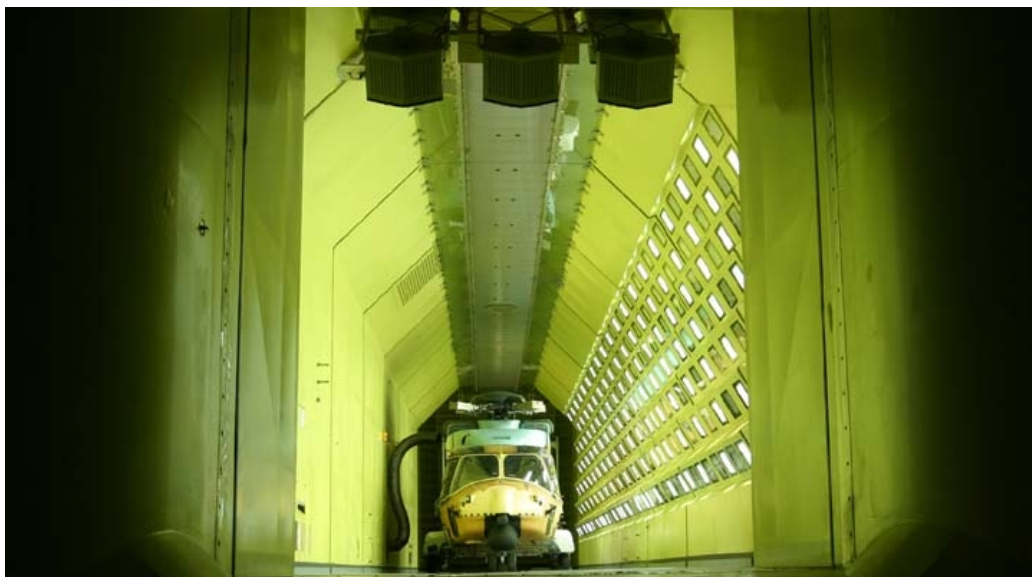
Figure 36 Helicopter in the Icing Wind Tunnel at the RTA (1)
